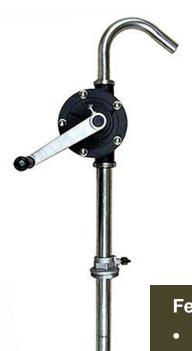
This is an advanced quality *Ryton Rotary Hand Pump* useful for most drums and tanks with a 2" Npt bunghole. Made from virgin grade oxidation resistant Ryton, Stainless Steel and PTFE. It can be mounted on 2" Npt bung holes of 15, 30, 55 gallon drums or bunged tanks.
